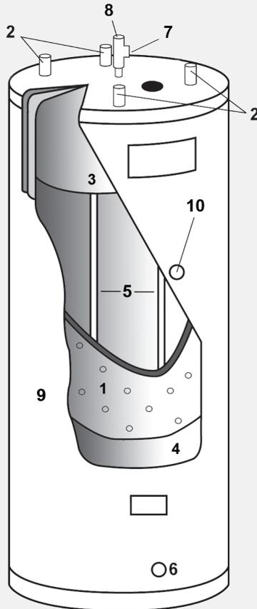
Therma-Stor plate design, with rapid, free-flowing paths for refrigerant gas, promotes excellent waste heat transfer throughout the tank.
